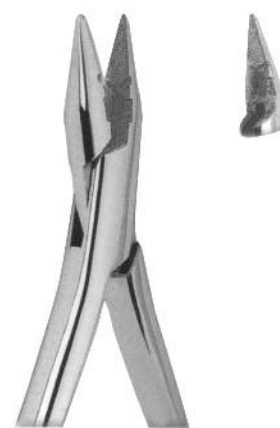
3216 Universal Universal pin roughening, cutting and bending pliers. For wires up to 0,9 mm. (.035"). Will cut wires up to 0,7 mm. (.028").
