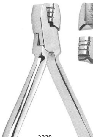
3220 De La Rosa De La Rosa arch forming pliers. Designed to form and contour arch wires on round or rectangular wire. The beak has grooves of 0,4 mm (.016"), 0,46 mm (.018") and 0,56 mm (.022").
